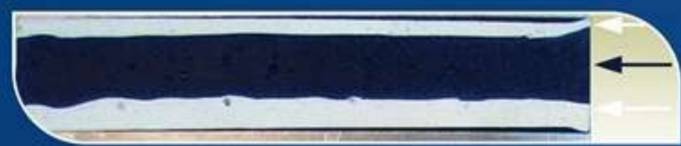
Mixing of blue and white resins in an empty pipe - Internal without any elements.
