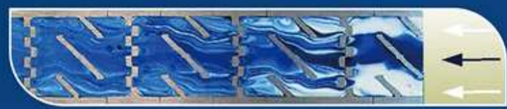
Mixing of blue and white resins in an empty pipe - Internal with SX model elements.
